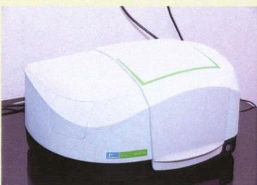
**Fourier-Transform Infrared Spectroscopy**
